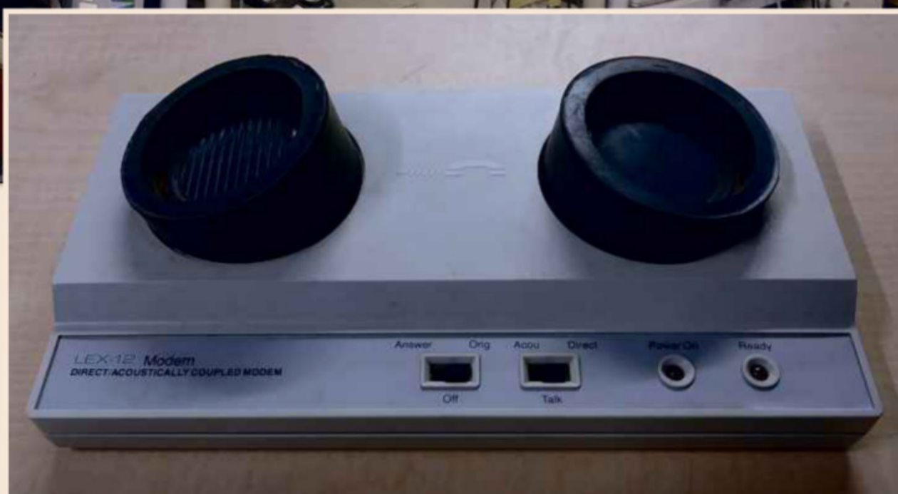
↑ This early modem from 1981 allowed direct coupling at the telephone handset jack, direct coupling to the phone line or acoustic coupling through the telephone handset
