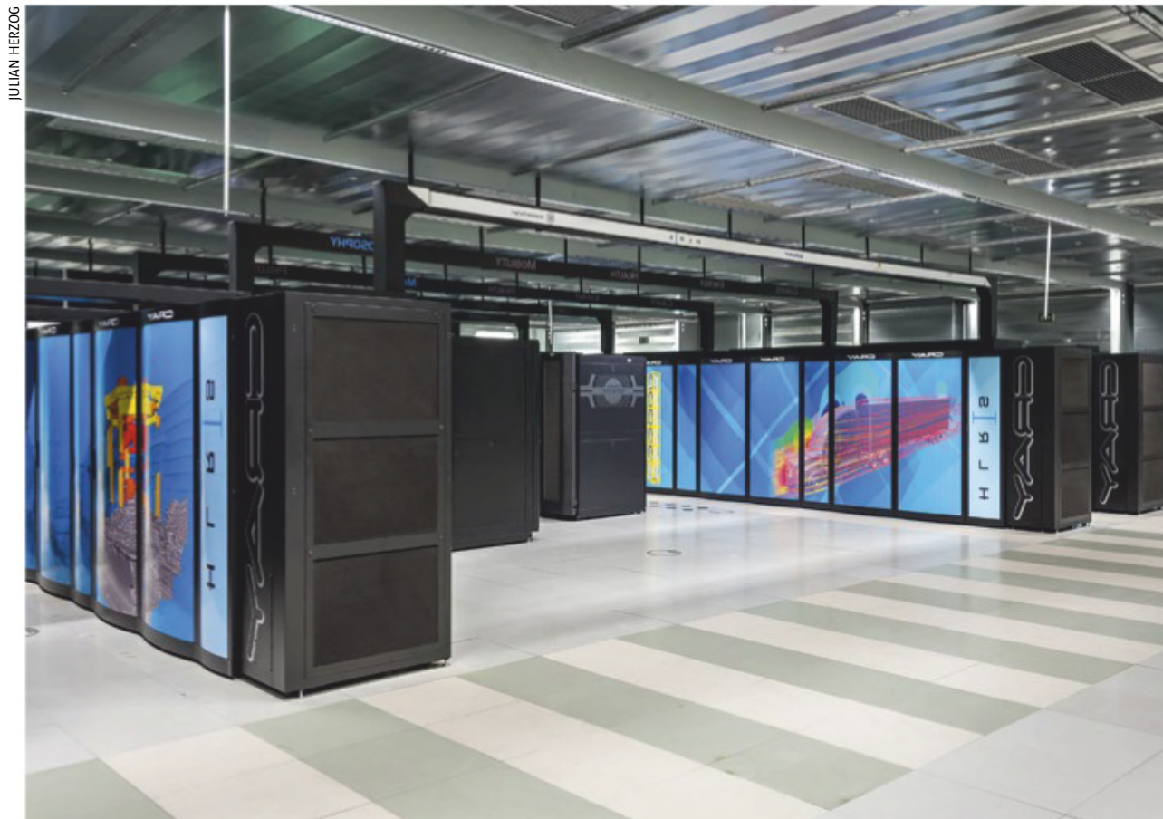
Global climate models require huge computing power, and are calculated by supercomputers such as this Cray XC40 in the University of Stuttgart, Germany. It can make 7.4 quadrillion calculations per second.
