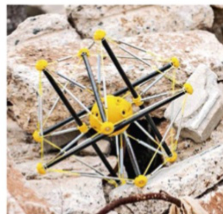
DROP & ROLL: Six shock absorbers protect the core of a new robot so it can survive falls from a great height.
