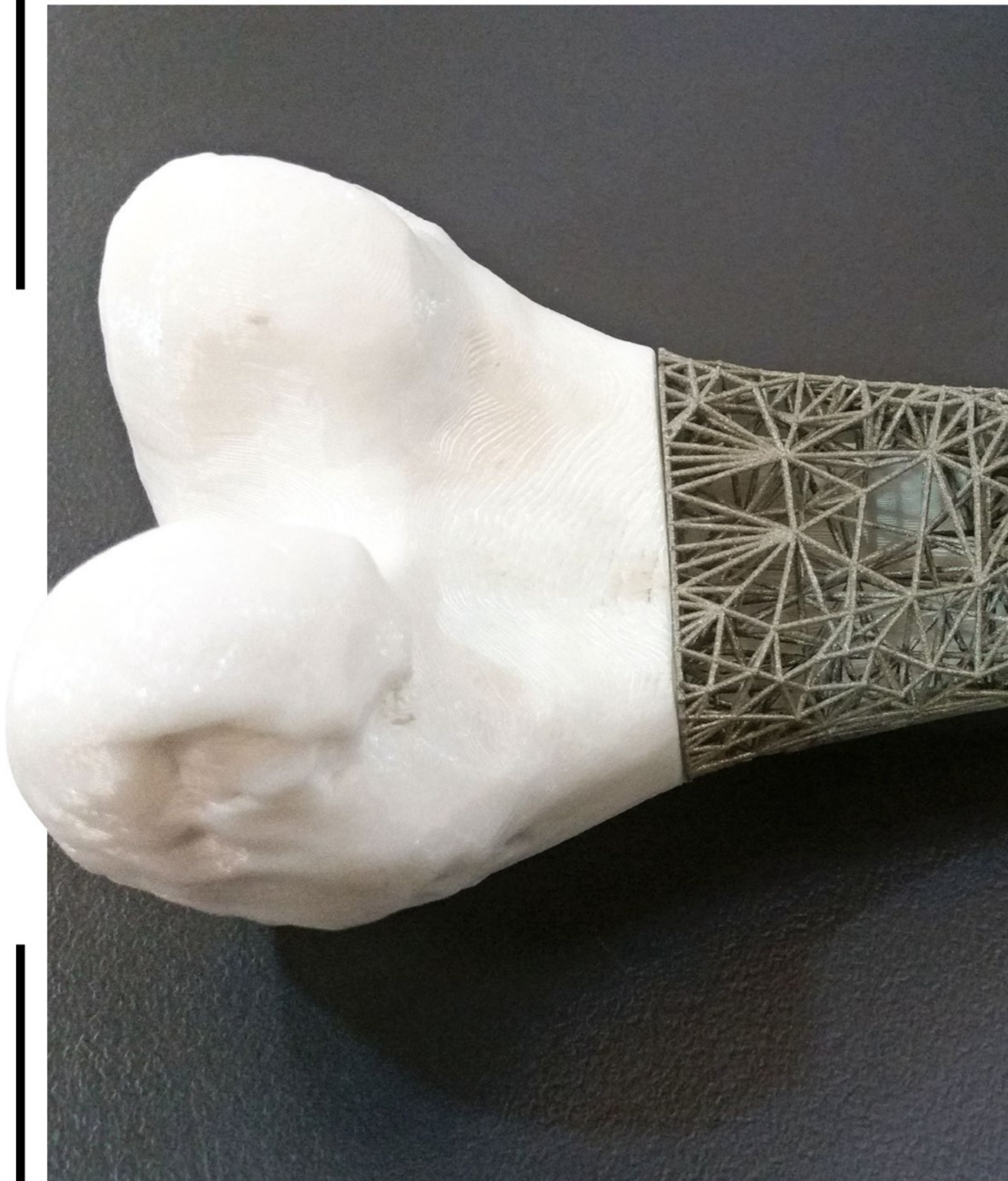
| BONE FILLING | Removed bone segments are replaced by 3D-printed copies.
