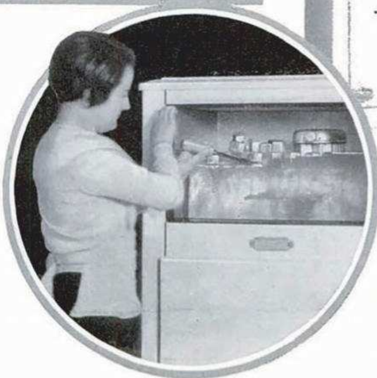
MAKING ICE CUBES Housewives who do not have automatic refrigerators can still have ice cubes with the aid of the device shown above. Filled with hot water and set on top of a block of ice, its cutting edges quickly sink into the ice. Then when it is lifted off, the cubes thus formed can be easily removed
